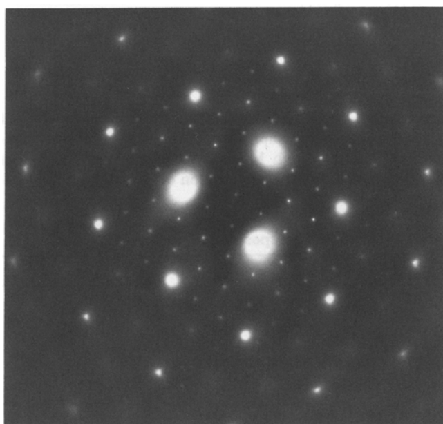
Fig. 2 Selected area diffraction pattern of the precipitate. Zone axis is \langle 111 \rangle .
